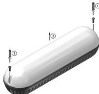
3. Release two screws (1) and remove assembly board / LED board (2) (avoid touching and damage to LEDs).
