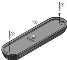
4. Put mains cable through bushing into luminaire body and strip it on 8 mm<sup>2</sup>.
