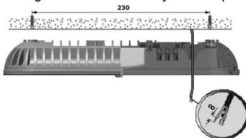
5. Attach the body to ceiling surface with X5 fasteners kit (not included), having put rubber washers (included) on screws beforehand. For luminaries with motion sensor mounting height is 1.5-3.5 m.
