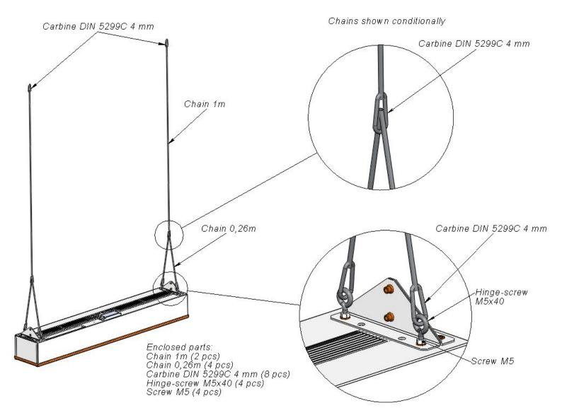
To adjust the luminaire height, if necessary, tighten M5 nuts (included in the delivery set) on the screws, thereby compensating the difference in the chains lengths
