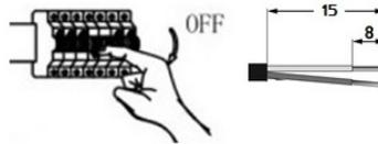
4. Connect mains cable to control gear's terminals according to scheme and polarity: "L" - phase conductor, "N" - negative conductor, the protective cover should be previously removed. Replace and secure control gear's protective cover.
