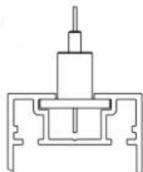
6.2. Place end cups and diffuser on the casing
