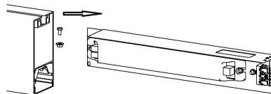
5. Put mains cable through opening in the casing and out from profile Connect mains cable to the control gear according to polarity shown, place the bracket with control gear back into the casing.
