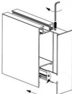
6.3. Attach suspension kit to bearing surface. Place ends of the wires into suspension grippers on luminaire's casing Adjust luminaire position.
