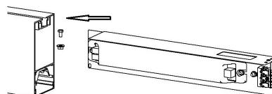
6. For installation of the luminaries to the rope suspensions:
