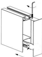
7.3. Using mounting holes, install the housing of the luminaire on the surface by means of self-tapping screws.
