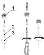
7. For installation of the luminaires on surface:
