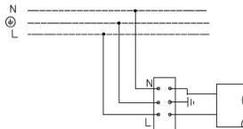
2. Mains connection scheme for luminaire with backup power supply: (on fig. a - luminaire, b - backup power supply unit).
