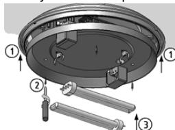
7. Replace the diffuser and fix it with screws.
