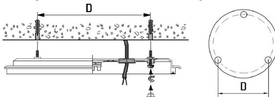
5. Connect mains cable to terminals according to polarity shown.
