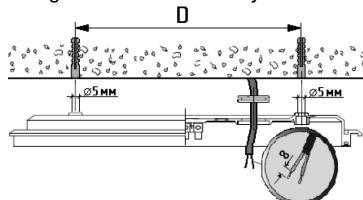
4. Place the body on ceiling surface. Insert stubs into mounting holes.
