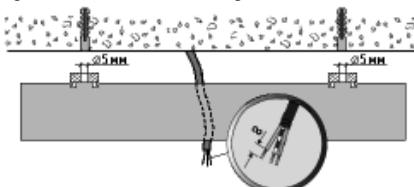
5. Connect mains cable to terminals according to polarity shown.
