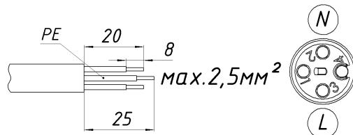
4. Lock wires with screws, assemble connector in reverse order. Bushings' tightening torque 2.5 Nm.
