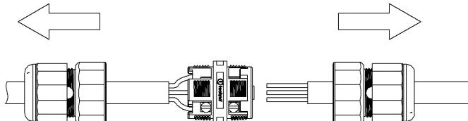
3. Strip the cable and connect it according to the scheme
