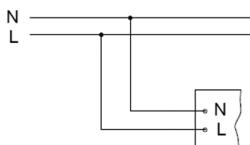
2. Mains connection scheme for luminaire with backup power supply: (on fig. a - luminaire, b - backup power supply unit).
