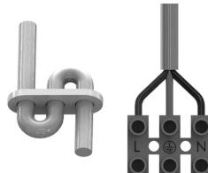
4. Install lamp. In K 200/209 luminaire lamps should have lamp manufacturer's permission to be used in serial connection to EmCG.
