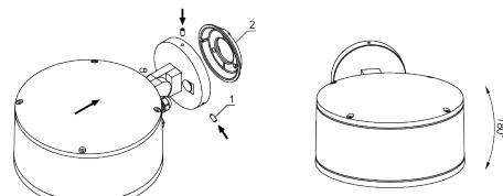
6. Release screws (6) and (7). Adjust luminaire position. Tighten screws (6) and (7).
