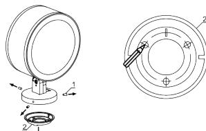
4. For hidden wiring remove plug (4) from rotary bracket (3) and place bushing (5) on its place, the busing is included in delivery set. Next put luminaire wire through the bushing (5).
