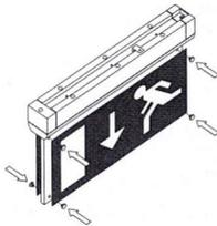
2. Place luminaire on a ceiling or a wall.
