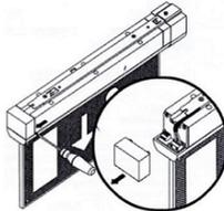
4. Switch mains power on and make sure the icons are glowing. Green LED battery charge indicator in the luminaire should also be on. For proper luminaire operation the battery have to be charged for 24 hours since it is delivered uncharged.
