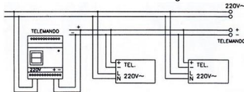
2. Connection scheme of luminaires for centralized mains power.
