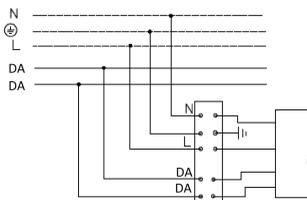
4. Mains connection scheme for luminaire with 1-10V dimmable driver.
