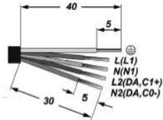
3. Connect mains cable to terminal block on back side of casing according to polarity shown. When regulated control gear is used, control wires connection polarity must follow label markings.
