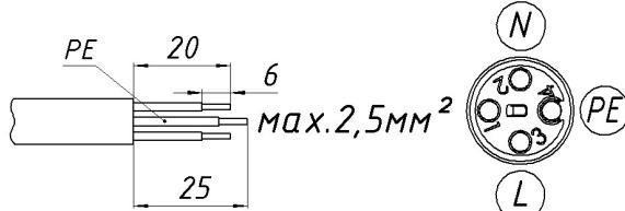
4. Lock wires with screws, assemble connector in reverse order. Bushings' tightening torque 2.5 Nm.
